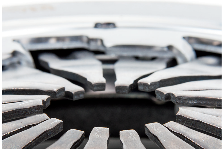
Fig. 1: Misalignment of diaphragm spring fingers on a dismantled clutch
