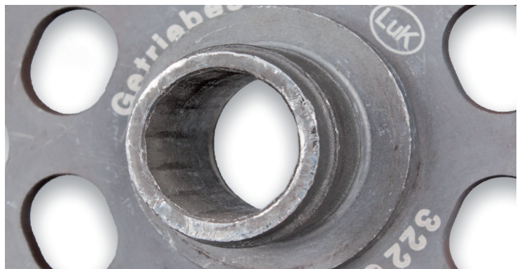
Image 2: Damaged spline profile
